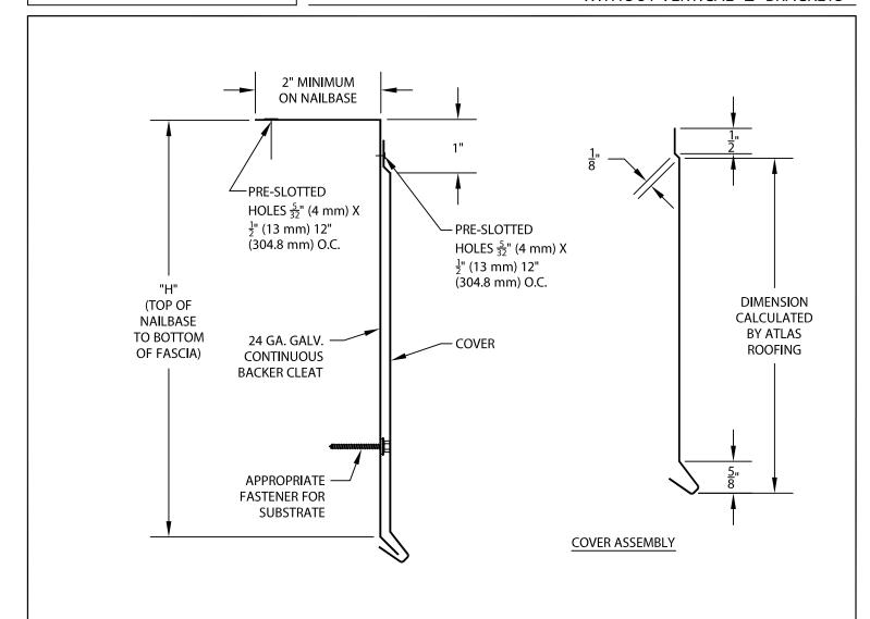
PANEL IS TO BE INSTALLED PER SPECIFICATIONS AND ATLAS ROOFING'S INSTALLATION INSTRUCTIONS DWG. # 38127-10910 NOTE: ALL FASTENERS BY OTHERS (SEE INSTALLATION INSTRUCTIONS FOR **RECOMMENDATIONS)**
